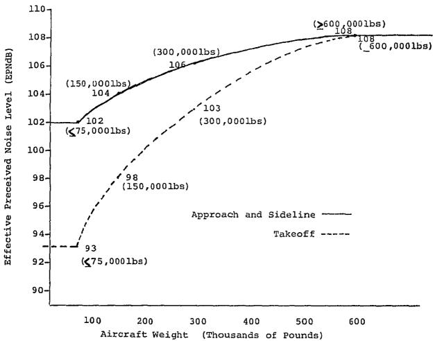
Many other factors such as weight of the aircraft, configuration of the flaps, and glide path are specified for the purposes of the testing. Note in the chart that two sideline measuring distances are shown. The .25 NMi distance applies to aircraft of less than four engines and the .35 NMi for the four or more engine category.
