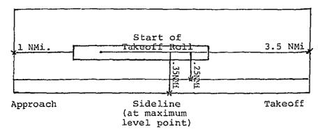
Using these measuring points, the aircraft type must be capable of limiting the noise generated according to the following graph:
